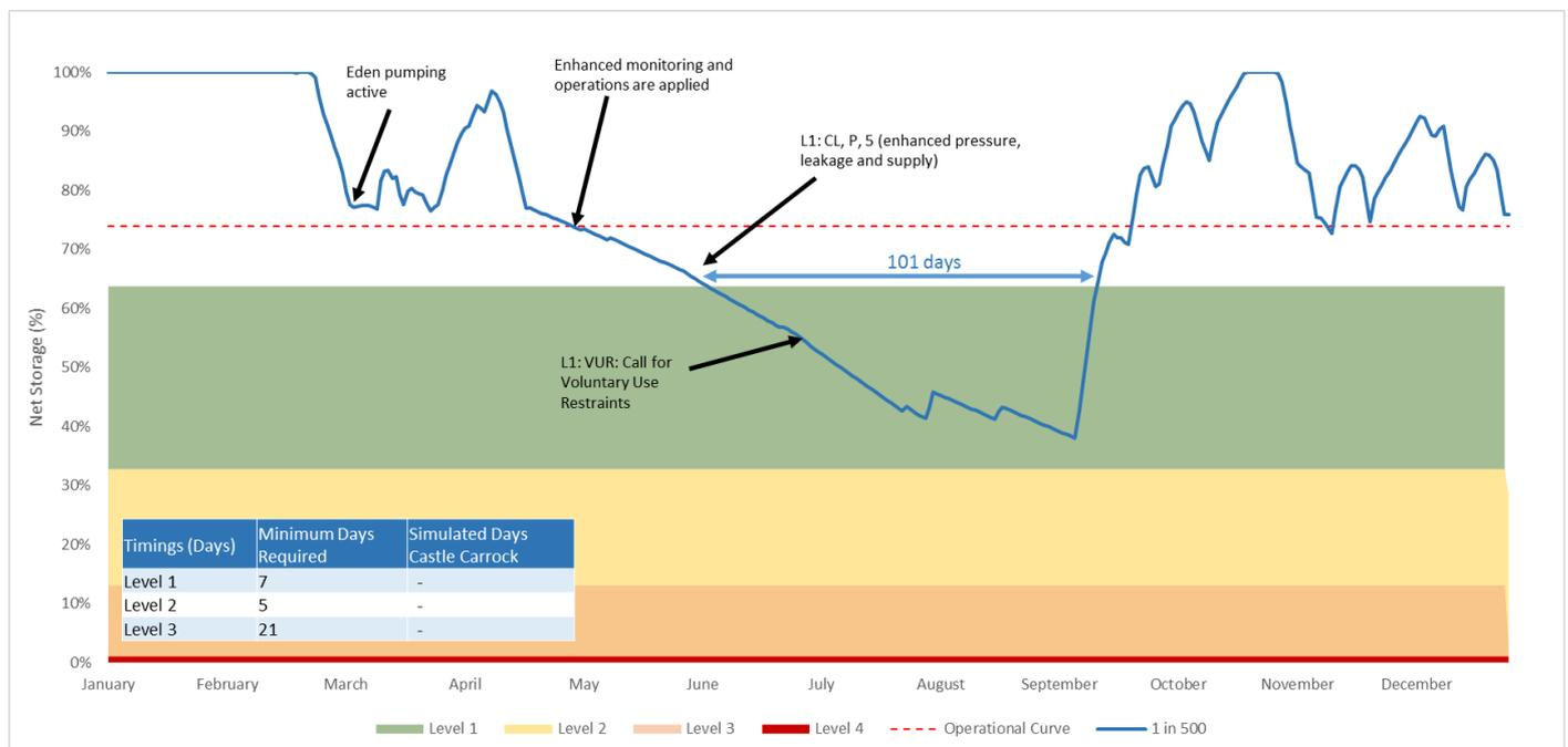
Figure 15 – Castle Carrock simulated storage, also showing new drought levels, salient drought and operational actions and timing between levels (inset table)
