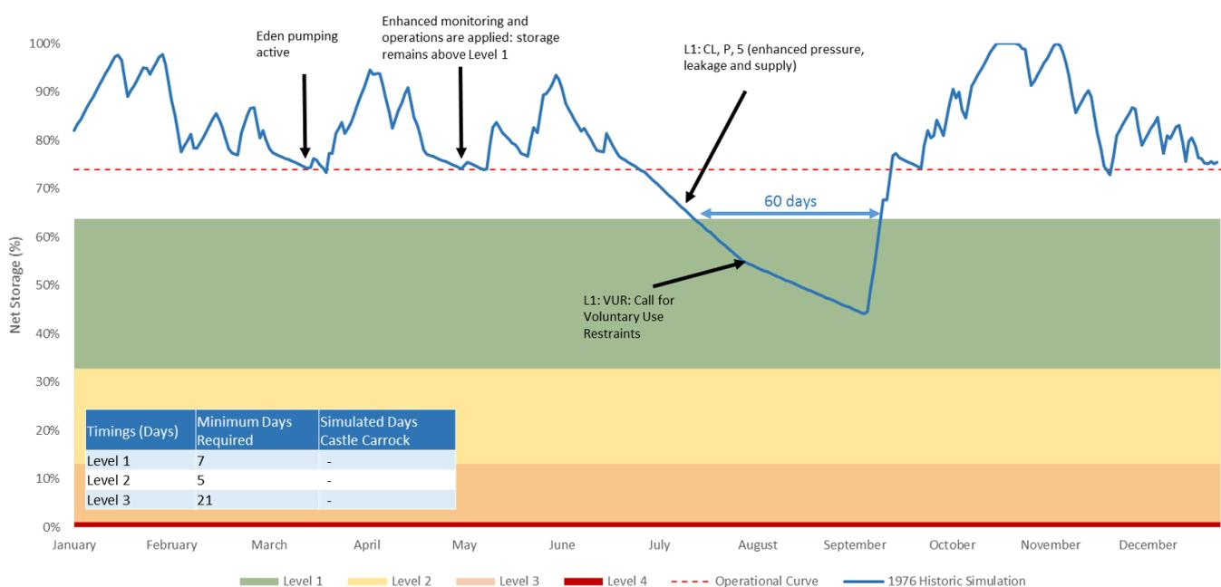
Figure 14 – Castle Carrock simulated storage, also showing new drought levels, salient drought and operational actions and timing between levels (inset table)
