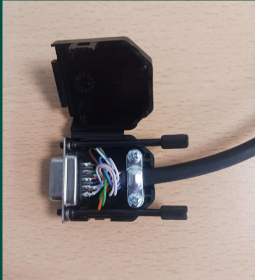
Modbus connections to APP and standard T4C RJ45
